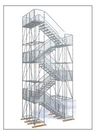
The Stairtower 500 is intended for temporary stairway structures with higher loads. It is preferably used as a site stairtower, e.g. for access to the site or as a road crossing not open to the public during construction work, but also at buildings as an additional escape stairtower. Under certain circumstances, the Stairtower 500 can also be used for public access during construction work or as a mandatory escape stairtower.
