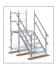
With the Layher modular stair, accesses can be constructed that always fit and match the system. Any intermediate dimension with a pitch of 20 cm can be achieved simply by fitting together the individual stairway parts. The top element is suspended in the U-section of either the assembly frame or the Allround ledger. At the bottom, the end section with scaffolding spindles is used for precise levelling.
