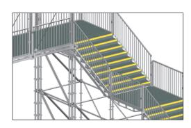
Sure footing with Layher step covers. With their non-slip surface using quartz sand, they ensure maximum safety on Layher stairs in rain, snow and ice conditions. The step covers are made from glass-fibre-reinforced plastic. They are permanently resistant to weather effects, easy to clean, electrically non-conductive and flame-retardant. They can be fitted quickly and are optimally matched to the Layher stair range.
