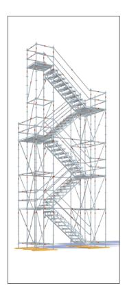
With the Allround site stairtower 200, 12-standard, each stair is assembled from 2 separate U-stair stringers 200 and 32 cm-wide standard decks used as steps. On the one hand this makes the weight/volume of the individual parts lower, the proportions of standard material higher, and the additional costs lower, and on the other hand it permits variable stair widths. Standard Allround diagonal braces are used as stair guardrails.
