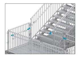
With the system handrail, complex one-off designs and assembly work can be avoided. With just three parts - handrail holder, joint and handrail tube - the guardrail can be installed quickly and easily for every stair type in line with regulations. The lightweight aluminium handrail tubes with dia. 42.3 mm for a pleasant grip are easy to cut and drill into and are also quick to clean. They are simply riveted to the fitted handrail holders.
