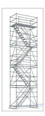
The Allround modular stairtower is the perfect solution for access to excavations, unfinished buildings and formwork at sites, and much more besides. Thanks to the 2.21 m-long Allround standard, the stairtower has no joint-overlapping components, and can be pre-assembled on the ground storey by storey and then emplaced by crane. Access is possible at both the ends and at the sides. You also have the benefit of 20 cm more headroom in a unidirectional stair than in a conventional one.
