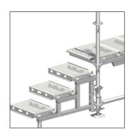
Adjustment to the ground, with access to the first scaffolding level, can be achieved with the Allround modular stair. The construction kit comprises: stringer for modular stair with 1, 2 and 3 steps, base collar for modular stair 0.26 m and O-ledger LW 0.90 m. 0.32 m-wide standard scaffolding decks in the selected length are installed as steps. The steps are fastened using lift-off preventers.
