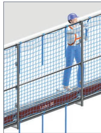
Fig. 13 Attaching the side protection net to the upper SpeedyScaf guardrail
