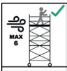
When used in the open air or in open buildings, **any work on the mobile platform must be stopped immediately if the wind strength exceeds 6 on the Beaufort scale.** At these wind speeds or at the end of a shift, mobile working platforms must be moved to a location where they are protected from the wind or must be or suitable measures must be taken to secure them against toppling over.
