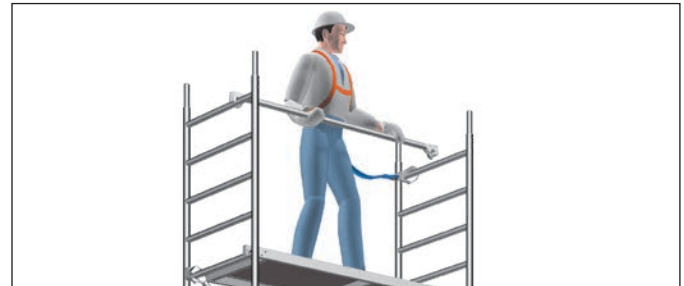
Fig. 3: Safe fitting of guardrail with PPE
