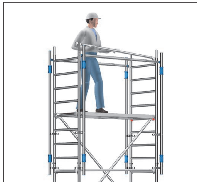
Fig. 6: Safe fitting of guardrails with AGS
