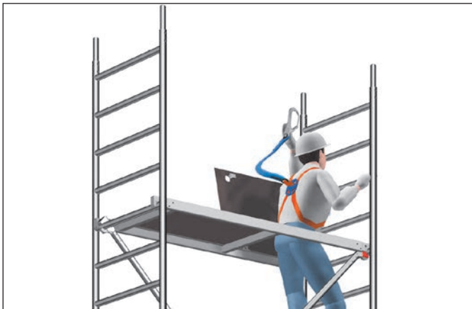
Fig. 1: Attachment of PPE during ascent to the unsecured level
