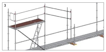
Swing it upwards, fit the AGS standard, install the U-ledger and insert the deck. The entire facade scaffolding can be safely assembled in the same way. Dismantling is in the reverse order.
