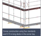
Correctly designed corners are a crucial factor for more safety when working. Advancing side protection in the corner and end bays is possible without the use of additional temporary components. The corner solutions shown here represent outside corners. Inside corners can be made in the same way. Non system bays at inside corners are accommodated by using the adjustable guardrails.
