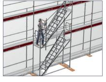
With the AGS System, external platform stairtowers too can be assembled with advancing side protection. Stair accesses are required by TRBS 2121-1 rules when the access height exceeds 5 metres.
