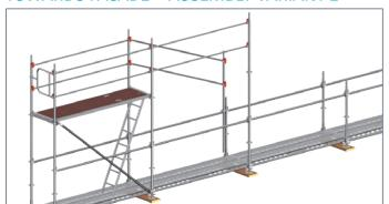
The AGS standard permits advancing guardrail fitting both on the outside of the scaffolding and on both sides. In this case, start with a 1-metre standard on the inside of the scaffolding towards the facade, in the same way as on its outside. Further fitting is done identically to assembly variant 1.
