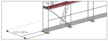
If larger work surfaces are required for reinforcing scaffolding, for example, the scaffolding width can be freely selected up to 3.07 m by using standard U-ledgers or O-ledgers.
