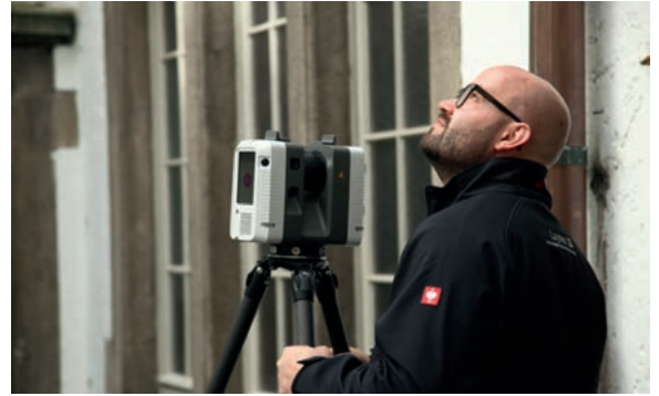
The mobile 3D laser scanner captures the building structure step by step.
