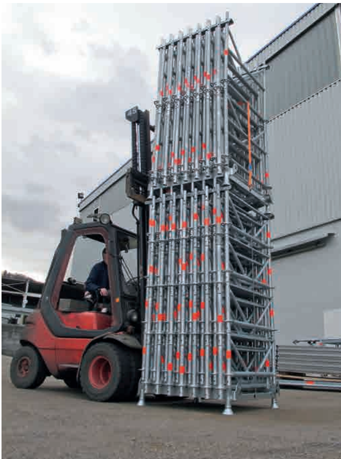
Filled and stacked TG 60 frame pallets for transport using a fork-lift truck
