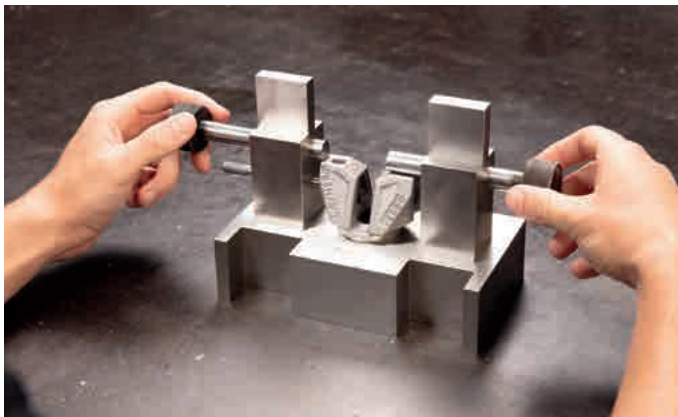
Dimensional and function test of the semi-finished parts
