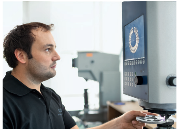
Hardness test during the incoming-goods inspection
